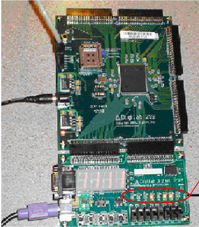
Fig. 4. Unidirectional PS/2 interface from keyboard to FPGA.
