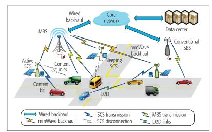
Figure 1. Vehicular network architecture with self-sustaining caching stations.
