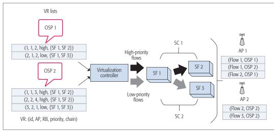
Figure 3. NSC example using the matching-theoretic OTT flow prioritization algorithm.
