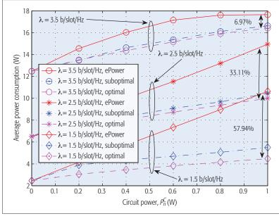
**Figure 4.** An example: average power consumption with the circuit power of each RRH, denoted by  $P_{n,r}^{c}$  under different traffic arrival rates  $\lambda$  in downlink H-CRANs, where a MBS, 8 RRHs, and 12 users are included. In this example, we formulate a network EE maximization problem that enfolds stochas tic and time-varying traffic arrivals to jointly optimize RRH operation and power allocation.
