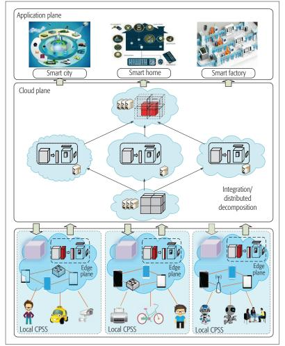
Figure 2. Cloud-edge computing framework.
