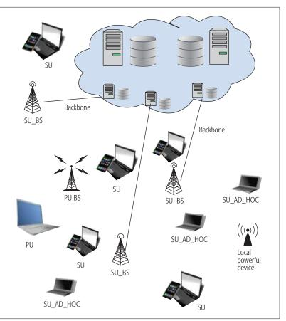
Figure 1. The cognitive radio network cloud.
