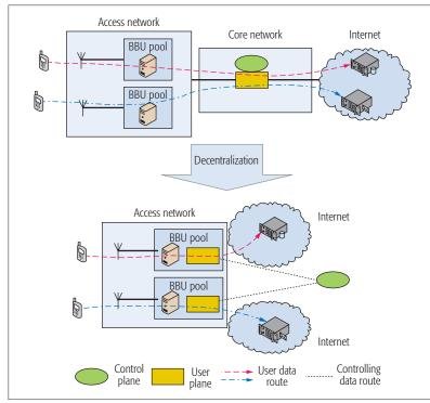
Figure 3. Evolution to the decentralized core network.
