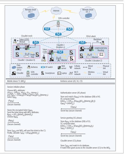
Figure 3. Mobile devices authentication at cloudlet mesh using Kerberos as a countermeasure for DDoS attack.
