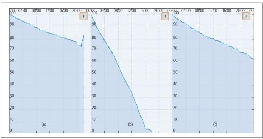
Figure 2. Battery drain experimental results (HYCCUPS Tracer screenshots). Axis X specifies the time of day, while axis Y is the device's battery percentage: a) regular power drain (no Wi-Fi Direct); b) continuously use Wi-Fi Direct; c) run Wi-Fi Direct for 1 minute every other 10 minutes.
