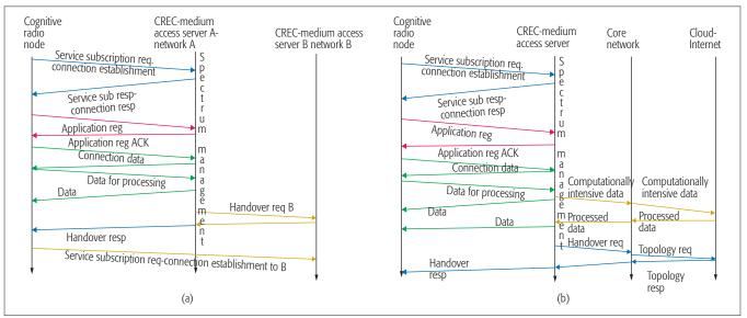
Figure 4. CREC- medium access server operating: a) at a powerful local node; b) on the RAN.
