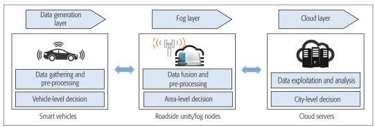
Figure 1. Architecture of vehicular fog computing.
