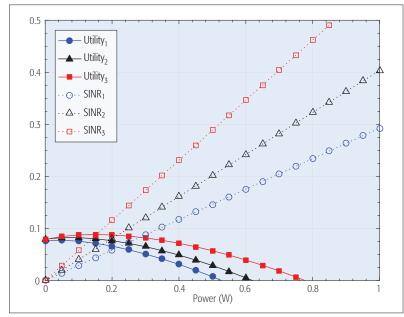
**Figure 2.** Correlations between  $U_i$  and  $p_i$ , and  $SINR_i$  and p.
