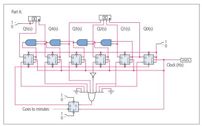
Figure 3. Digital circuit inside of part A; this circuit counts the seconds.
