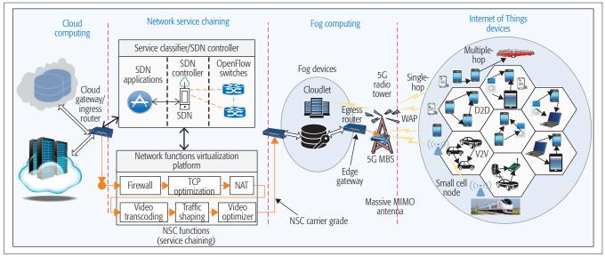
Figure 2. Network service chaining model in 5G wireless architecture.
