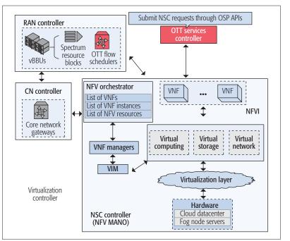
Figure 2. SDN/NFV framework for OSPs' NSC.
