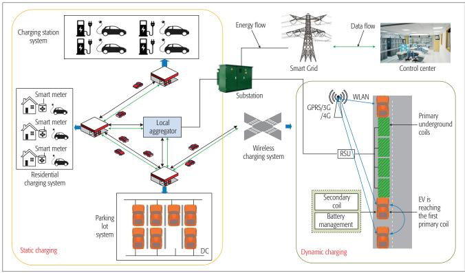
Figure 1. The structure of an EV charging network.
