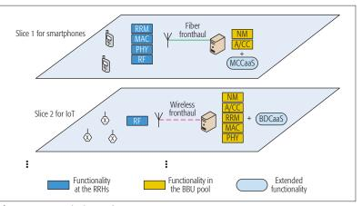
Figure 6. Network slicing for C-RAN.
