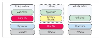
Figure 2. VMs vs. containers vs. UniKernels.
