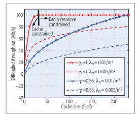
Figure 4. Service capability of SCSs with different cache sizes.
