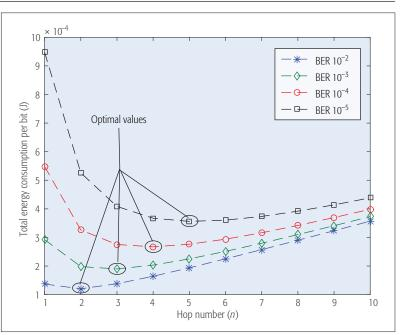
Figure 5. Optimal number of hops vs. energy consumption.
