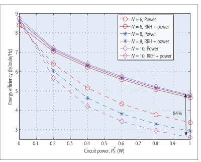
**Figure 2.** An example: EE variation with the circuit power of each RRH, denoted by  $P_n^c$ , in downlink H-CRANs, where an MBS, *N* RRHs, and 16 users are included. In this example, we maximize the network EE by optimizing RRH operation and power allocation subject to constraints of users' minimum rate requirements of  $R^{\text{req}} = 2 \text{ b/Hz}$ .
