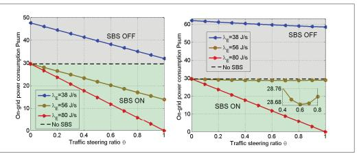
Figure 4. Power consumption with respect to traffic steering ratio: a) on-grid EH-SBS; b) off-grid EH-SBS.
