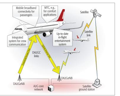
Figure 1. Structure of A2G communication including DA2GC and SC with services available for onboard passengers, crew and MTC.
