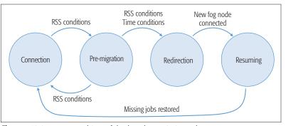
Figure 4. Finite state machine of the handover timing scheme.
