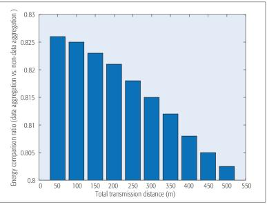
Figure 2. Energy comparison over transmission distance.
