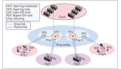
Figure 3. System architecture with active HFog overlays.
