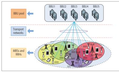
Figure 1. The architecture of H-CRANs.
