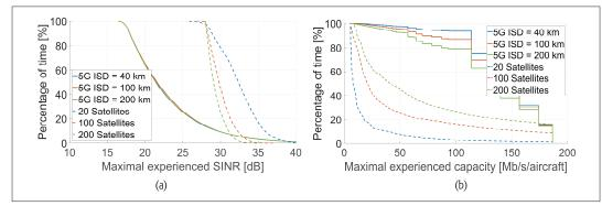
Figure 3. a) Maximal average SINR; b) capacity experienced by aircraft over flight duration for 5G DA2GC network and satellite communication.
