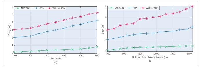
Figure 4. Results obtained with/without SDN and NSC-SDN approaches: a) delay vs. user density; b) delay vs. distance between user and destination.
