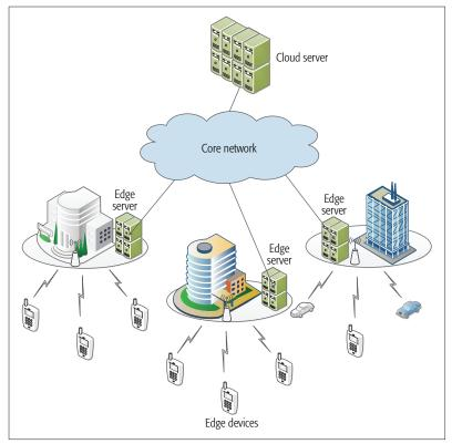
Figure 1. Edge-fog-cloud computing architecture as an ecosystem of different cyber-physical systems.
