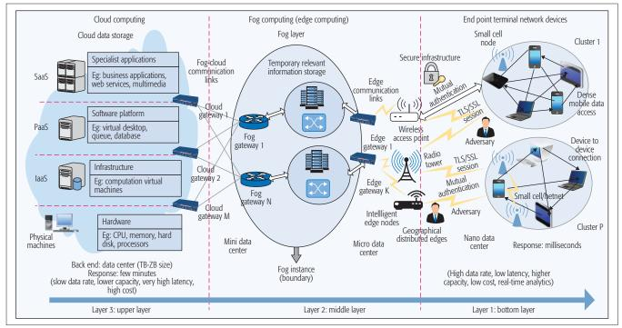
Figure 1. Detailed system architecture for integration of cloud, fog, and end point terminals.
