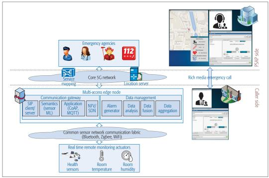
Figure 3. MEC-enabled emergency call component diagram.
