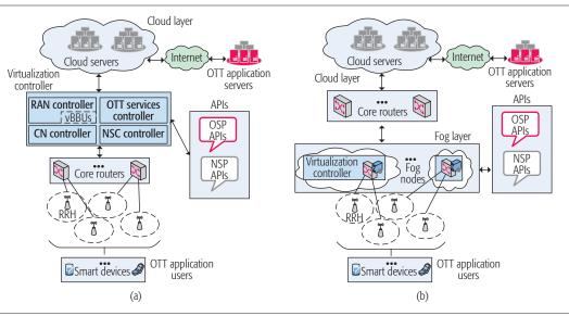
Figure 1. Network management architectures for OSPs: a) cloud-based architecture (C-RAN); b) fog-based architecture (F-RAN).
