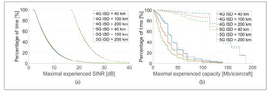
Figure 2. a) Maximal average SINR; b) capacity experienced by aircraft over flight duration for 4G and 5G DA2GC networks.
