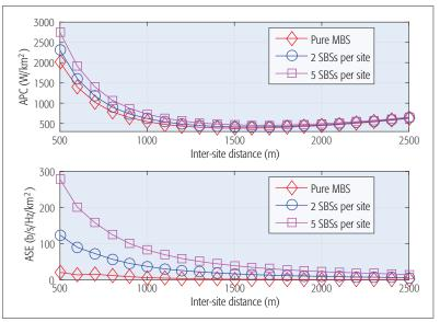
**Figure 3.** An example: The APC and ASE vs. the inter-site distance subject to a 95 percent coverage constraint. In the figure, we adopt the practical models for the BS power consumption given by  $P^{\text{tot}} = ap^{\text{tx}} + b$ , where  $a_{\text{MBS}} = 22.6$ ,  $b_{\text{MBS}} = 412.4$  W,  $a_{\text{SBS}} = 5.5$ , and  $b_{\text{SBS}} = 32$  W (note that SBSs refer to micro BSs in the figure) [15].
