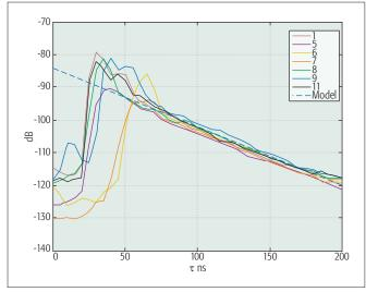
Figure 9. The average power delay profiles vs. delay in nanoseconds for different positions in an 11 m  $\times$  19 m furnished room. The dashed line is the theoretical reverberation model: frequency 5.8 GHz, bandwidth 100 MHz [20].
