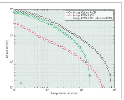
Figure 4. Payload size (device-specific information) versus arrival rate performance for one-stage and two-stage transmission strategies, 10KHz bandwidth, 1 second latency.
