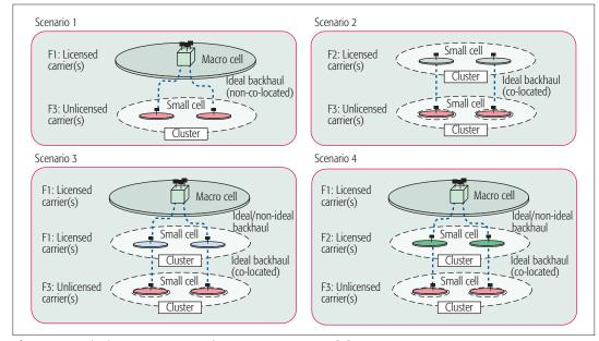
Figure 1. LAA deployment scenarios from 3GPP TR 36.889 [1].
