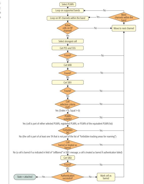
Figure 1. Initial cell selection process for the UE.
