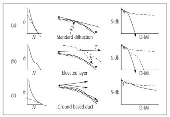
Figure 3. Tropospheric propagation mechanisms for various values of refraction index *N*. *D* is distance, *h* height [8].
