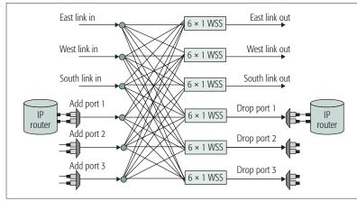
Figure 2. An IP router, which interfaces to add/drop port 1, wants to establish a connection on the East and West links. If  $\lambda 1$  is the only available wavelength on both of these links, one of the connections will be blocked due to wavelength contention on the add/drop port.
