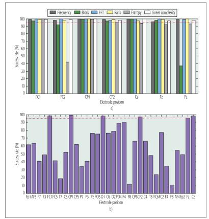
**Figure 3.** NIST test results: a) detailed results of the NIST tests for the electrodes in the Cz/Fz zone and surrounding area; b) mean success rate of the electrodes for the most three demanding NIST tests (frequency, block, and entropy). The red line is the NIST threshold of success.
