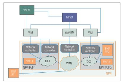
Figure 2. ETSI NFV Architecture (ETSI GS NFV-MAN 001 V1.1.1).
