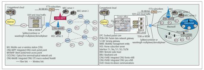
Figure 3. MEC over FiWi network architectures: a) MEC over Ethernet-based FiWi networks and MEC over 4G LTE-based FiWi networks; b) coexistence of MEC and C-RAN over FiWi enhanced 4G LTE HetNets.
