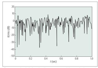
Figure 6. Rayleigh fading for *f* =900 MHz and for a vehicle speed of 120 km/h.
