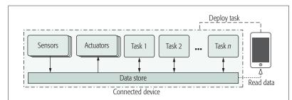
Figure 1. Tasks interacting in a loosely coupled manner.
