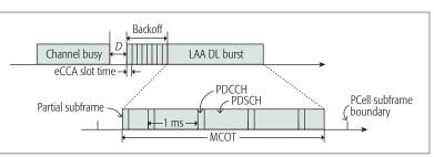
Figure 3. Illustration of an LAA DL burst transmission.
