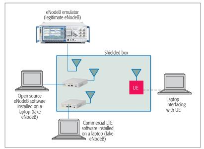
Figure 3. Block diagram of the testbed.
