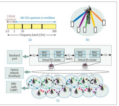
Figure 2. 5G C-RAN with mmWave and massive MIMO.
