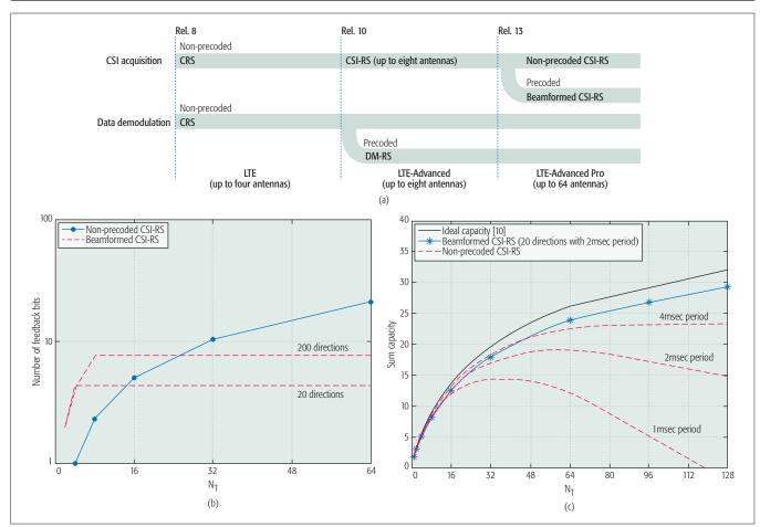
Figure 1. MIMO evaluation: a) RS evolution in LTE systems; b) uplink feedback overhead (SNR = 10dB [7]); c) MU-MIMO capacity with considering CSI-RS overhead (ideal CSI and ZFBF MU-precoding with 10 UEs and SNR = 10dB).
