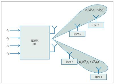
Figure 2. An illustration of NOMA with beamforming.
