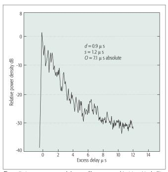
Figure 7. Average power delay profile measured in New York City [14] by Cox in 1975. The frequency is 910 MHz.
