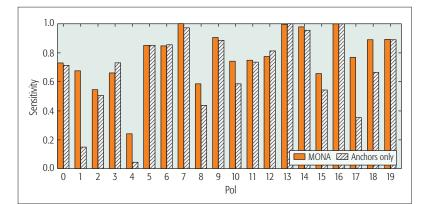
Figure 4. Positioning accuracy of our system with MONA and without it during the real-world experiment. Only Pols 7, 9, 13, 14, 16, and 19 were instrumented with an anchor. The average sensitivity was 0:68 and 0.77, respectively.
