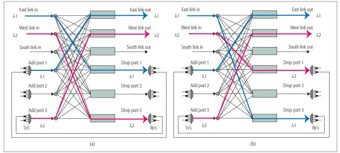
Figure 5. Shared restoration where pre-lit segments are concatenated to form the restoration path. Two pre-lit segments are shown, one on  $\lambda 1$  and one on  $\lambda 2$ : a) the configuration prior to failure; b) the desired configuration after a failure occurs, where the  $\lambda 1$  segment must be concatenated to the  $\lambda 2$  segment. To support this operation,  $\lambda 2$  must be available on drop port 1 and  $\lambda 1$  must be available on drop port 3.
