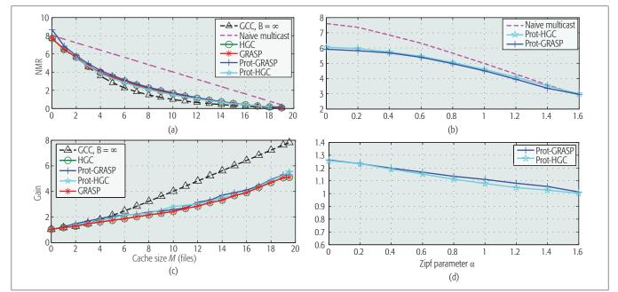
**Figure 5.** Comparison of the total minimum rate normalized by the one-user network minimum rate with respect to: a) the cache size with  $\alpha = 0$ ; b) the Zipf  $\alpha$  parameter with M = 2 files; and the gain of the coded over the uncoded scheme with respect to: c) the cache size with  $\alpha = 0$ , and d) the Zipf  $\alpha$  parameter with M = 2 files.
