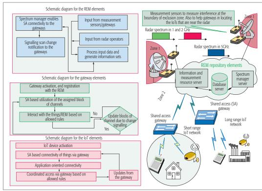
It is good for our proposal that the unlicensed bands are close to/adjacent to several radar bands. There are already IoT devices that are operating in different unlicensed frequency spectrum. This means that basically the same front end with some modifications can be used for our proposed framework.
