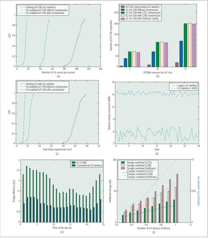
Figure 5. Simulation results showing uplink access, IoT GW capacity, latency dynamics, energy consumption, energy dynamics, and overhead: a) uplink access distribution; b) device capacity of cells; c) delay experienced by IoT-enabled devices; d) improvement in energy consumption; e) energy efficiency using C-RAN; f) traffic and computation overhead.
