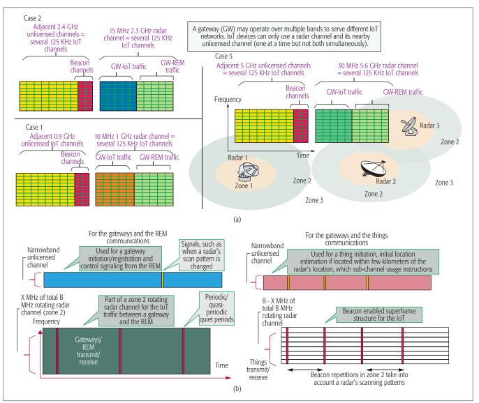
Figure 5. Examples of beacon and traffic channel blocks for the proposed SA for IoT devices.
