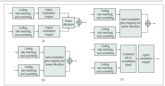
Figure 6. Examples of transmitter processing of candidate MUST schemes: a) MUST Category 1; b) MUST Category 2; c) MUST Category 3.
