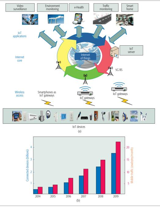
Figure 1. IoT architecture with connectivity and traffic forecast: a) IoT architecture involving IoT-gateways and 5G BS; b) forecast of mobile devices and traffic.
