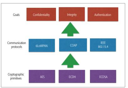
Figure 2. Current cryptographic primitives for securing communication in the loT.
