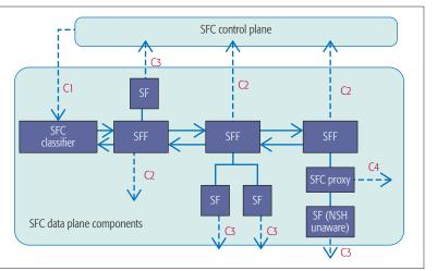
Figure 1. A typical SFC architecture (draft-ietf-sfc-control-plane-06).
