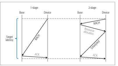
**Figure 3.** Schematics of one-stage and two-stage protocols. In the one-stage protocol, the device ID and data payload are transmitted on the uplink RACH, possibly resulting in a collision. In the two-stage protocol, the device ID is transmitted on the RACH. Following a downlink resource allocation, the data payload is transmitted on scheduled resources.
