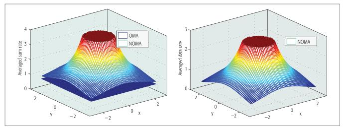
**Figure 5.** Performance of downlink NOMA transmission – an example. The transmit SNR is 20 dB. A fixed power allocation policy,  $(a_A, a_B) = (7/8, 1/8)$ , is used in the first subfigure. The power allocation coefficient used in the second figure needs to satisfy a targeted data rate of 0.5 BPCU at the primary user. The other parameters are set the same as in Fig. 4: a) fixed power allocation; b) cognitive radio power allocation.
