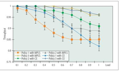
Figure 3. Throughput as a function of load for different policies.
