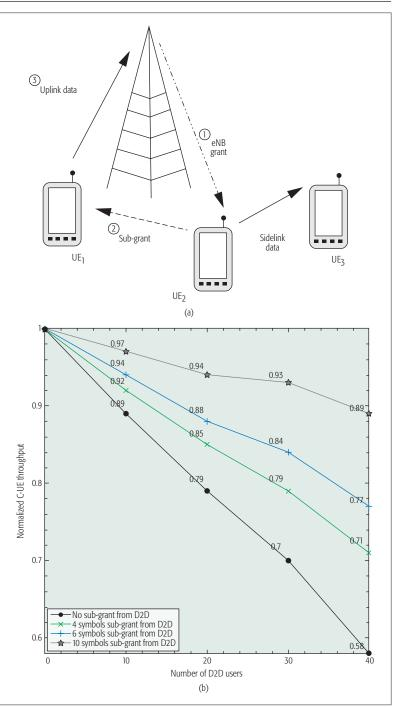
Figure 2. a) UE2 delegates its unused uplink resources to UE1; b) simulations show that in the investigated scenario with, for example, 20 devices delegating 4 OFDM symbols per sub-frame to some other devices, uplink throughput can be increased by 6 percent. More generally, the gain increases with the number of devices and the size of the sub-grant in this setting. Details may be found in [4].
