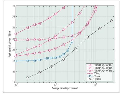
Figure 1. Peak transmit power versus arrival rate performance for RACH transmission strategies, 100KHz bandwidth, 1 second latency, 500 bit payload per device.
