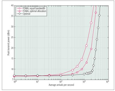
Figure 2. Peak transmit power versus arrival rate performance for scheduled transmission strategies, 100KHz bandwidth, 1 second latency, 500 bit payload per device.
