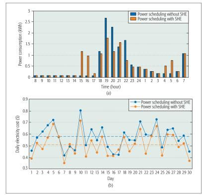
Figure 4. The results of power scheduling: a) hourly power consumption of a typical day; b) daily electricity cost of a month.
