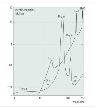
Figure 5. Atmospheric attenuation vs. frequency [10].
