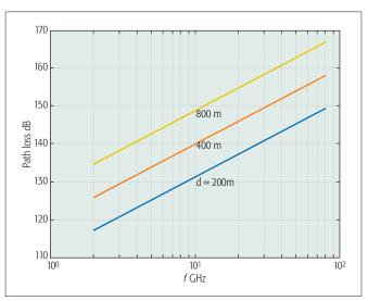
Figure 8. Path loss vs. frequency for a non-line-of-sight urban case, based on [16]. The slow fading is not shown.
