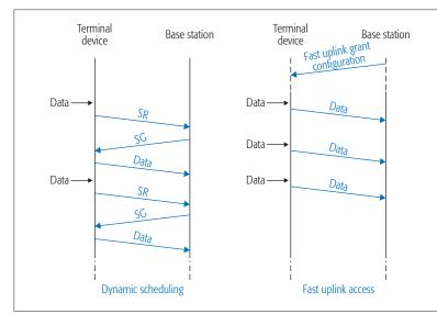
**Figure 3.** Message sequence chart for the dynamic scheduling and fast uplink access schemes. Dynamic scheduling imparts extra signaling delays due to the exchange of scheduling request (SR) and scheduling grant (SG) messages after data has arrived at the device. In fast uplink access, a BS configures the uplink resources in advance, and after the data arrives, it can be directly transmitted without explicit SR/SG exchange.
