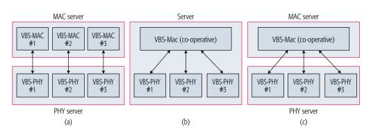
Figure 4. Split-VBS architectures: a) One-to-One mapping between PHY and MAC (different servers); b) Many-PHY-to-One-MAC (one server); c) Many-PHY-to-One-MAC (different servers). Note that the architectures in (a) and (c) (multi servers) can exploit the heterogeneity in datacenter server hardware.
