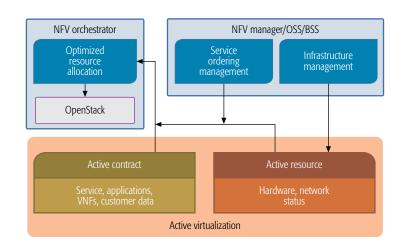
Figure 2. CloudNFV Architecture.
