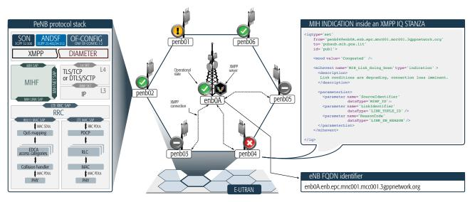
Figure 4. An instance of PeNBs deployed within the coverage area of an eNB.
