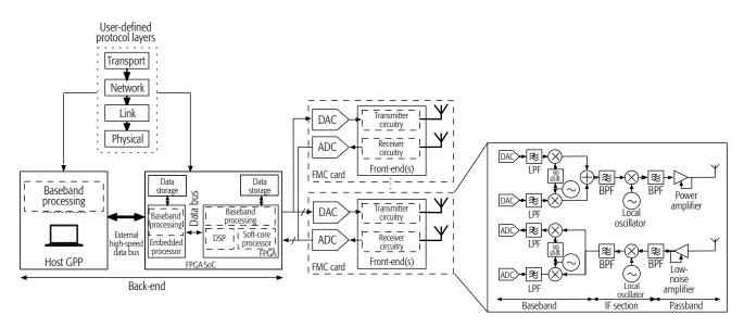
Figure 1. Generic software-defined radio architecture. Static analog transmit/receive circuitry (front-end) is interfaced with programmable hardware processing platforms (back-end) through ADCs/DACs. Analog-to-digital converters (ADCs)/digital-to-analog converters (DACs) and analog front-end radio circuitry may be featured under the same compact card, referred to as an FPGA mezzanine card (FMC).
