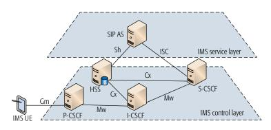
Figure 1. Simplified IMS architecture.
