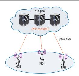
Figure 1. Cloud radio access network architecture, where the base stations are physically unbundled into virtual base stations and remote radio heads. Virtual base stations are housed in centralized processing pools and can communicate with each other at gigabit-per-second speeds.
