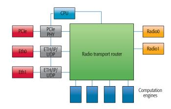
Figure 2. Schematic of the Ettus USRP E300 architecture.
