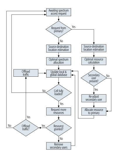
Figure 3. Resource management process at the BS. The proposed algorithm minimizes the dependence on spectrum sensing by relying on database assisted spectrum management.
