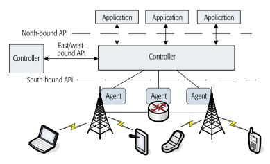
Figure 2. The conceptual architecture of SDWN.
