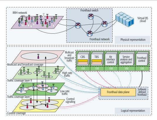
Figure 1. Software-defined hyper-cellular architecture.
