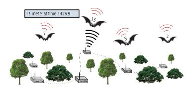
Figure 1. Conceptual scenario for bat tracking in the wild: stationary ground nodes are used to localize and track bats based on emitted beacon messages. The mobile nodes are also used to monitor encounters and download this data to the ground network to increase the observation range beyond the ground station area.
