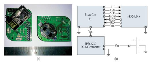
Figure 1. nRF24Cheep: custom designed BLE Beacon platform. The major components include: RL78-G14 microcontroller, NRF24L01 + 2.4 GHz RF transceiver, TPS62730 synchronous step-down DC-DC converter, and CR2032 battery holder. a) platform overview; b) functional representation of the major platform components.
