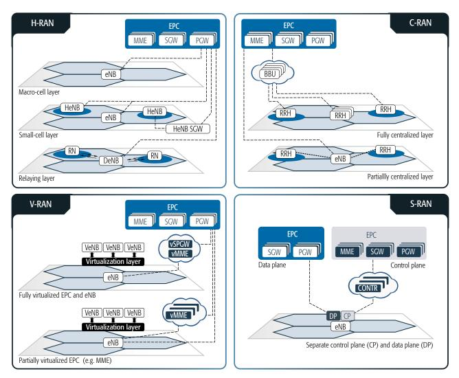
Figure 1. Mobile network architectures enabled by LTE. Heterogeneous radio access networks (H-RAN); centralized radio access networks. (C-RAN); virtual radio access networks (V-RAN); and software-defined radio access networks (S-RAN).
