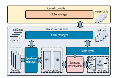
Figure 2. SDWN-enabled system architecture for spectrum management.
