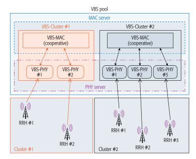
Figure 5. VBS-Cluster with a many-PHY-to-one-MAC architecture: VBSs associated with a cluster are merged together in the VBS-Cluster, and RRHs' antennae in each cluster act as a single coherent antenna array distributed over the cluster region.
