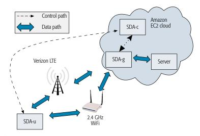
Figure 5. SDA-as-a-service experimental setup.
