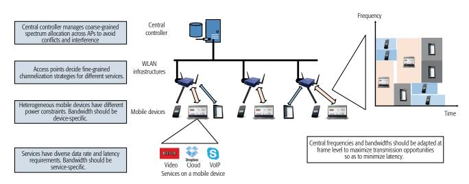
Figure 1. Illustration of fine-grained spectrum management.
