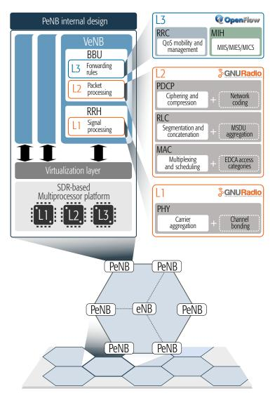
Figure 5. Internal design of PeNBs.
