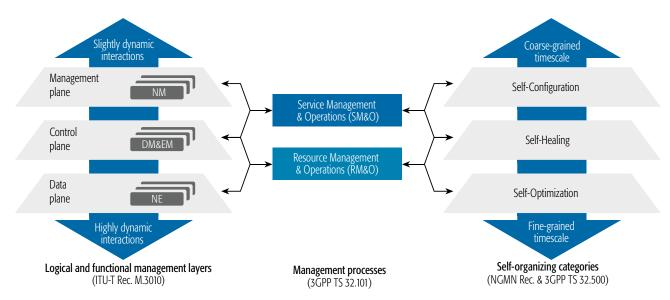
Figure 2. Functional layered networks.
