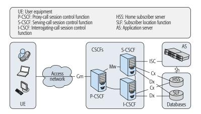
Figure 1. Simplified overview of the IMS architecture.
