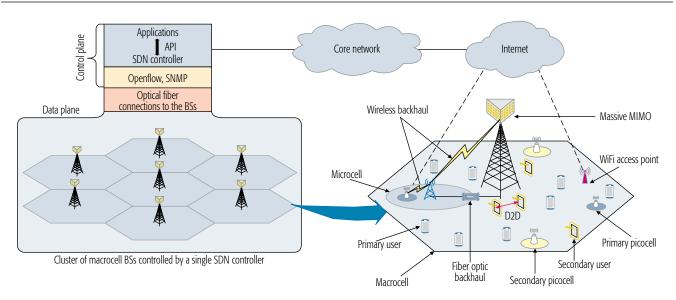
Figure 1. Software-defined 5G HetNet architecture that supports HSA. The macrocell BSs are directly connected to the controller, while the BSs of the smaller cells connect with the macrocells through a reliable backhaul link.
