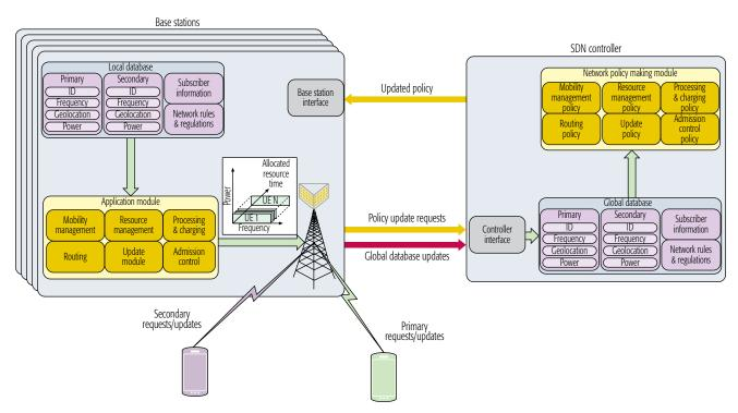
Figure 2. Operational architecture of the software-defined cellular network. The SDN controller decides the policies related to various network functionalities while the BSs implement the controller-defined policies.
