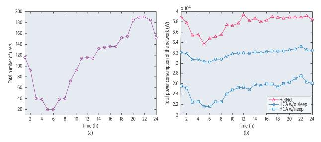
Figure 2. Simulation comparison of the network power consumption: a) average total number of users in the network for each hour; b) average total network power consumption for each hour.
