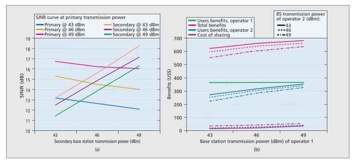
**Figure 4.** Cellular-cellular sharing scenario: a) average SINR of the primary and secondary users as the function of transmit powers of primary and secondary base stations; b) profits of the two sharing operators, individually and combined.
