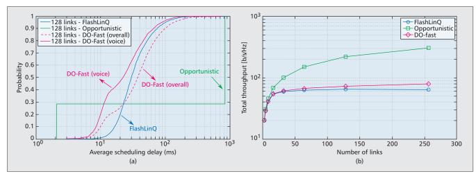
Figure 2. Simulation results: a) CDF of average scheduling delay; b) system throughput.
