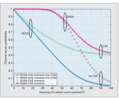
Figure 3. Channel access probability for a D2D TX vs. spatial intensity of cellular users for DUSA and DASA policies (with and without cognition).
