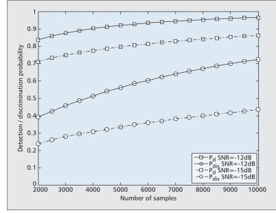
Figure 3. The theoretical performance metric of cognition vs. number of samples with system parameters known a priori.
