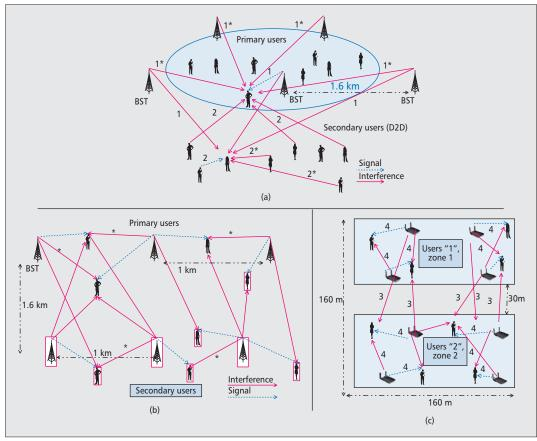
**Figure 2.** Three considered scenarios: a) FDD downlink transmission with D2D communication; the numbers above the arrows define the type of path loss models used: 1. COST Hata model, 2. ITU-R P.1411 end; b) cross-operator spectrum sharing; c) indoor-indoor co-primary sharing with the following path loss model: 3. In-building propagation model of [11, Eq. 5] with wall penetration loss: 4. In building propagation model path loss model.
