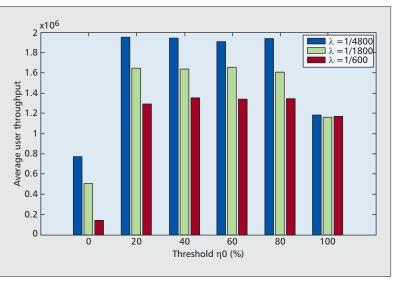
Figure 6. Average user (including blocked and unblocked) throughput in LTE-CR.
