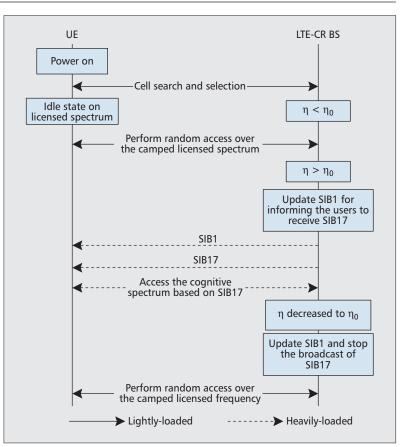
Figure 3. SIB-CPC-based backward-compatible network access.
