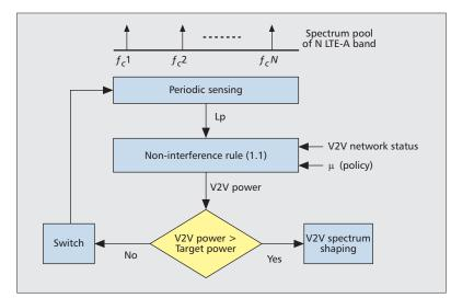
Figure 5. LTE-A spectrum pool mechanism..
