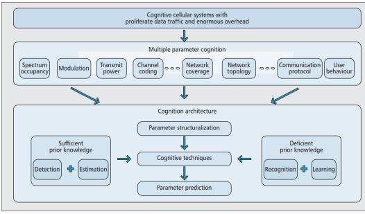
Figure 2. Framework of the multi-parameter space cognitive architecture.
