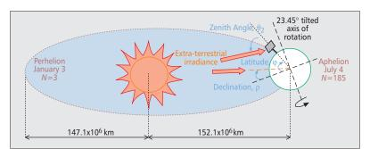
Figure 2. Illustration of the geophysical parameters controlling irradiance.
