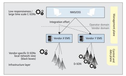
Figure 1. Typical positioning of SON functions in the control and management planes.
