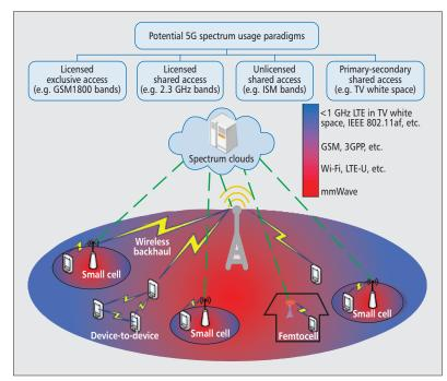
Figure 6. A vision for potential 5G spectrum usage paradigms.
