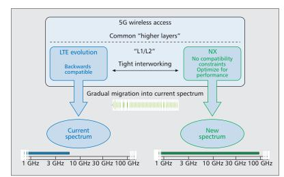
**Figure 1.** 5G wireless access in relation to spectrum. (Source: Ericsson white paper on 5G radio access.)
