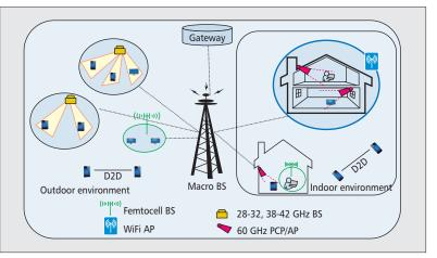
Figure 1. A 5G scenario with multiple radio access technologies.
