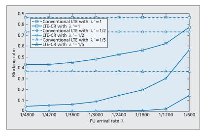
Figure 4. Blocking ratio with 10 TV channels ( $\mu = 1/1200, \mu' = 1/150$ ).
