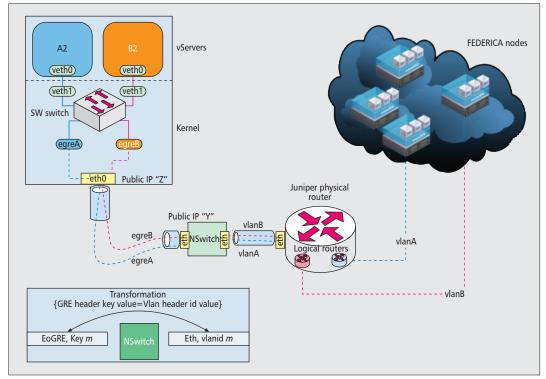
Figure 5. L2 network federation example of heterogeneous virtual infrastructures (GRE & 802.1q protocols are used for L2 topology creation).
