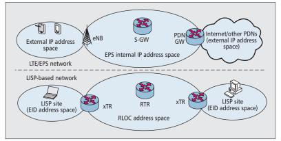
Figure 1. IP addressing architecture of LTE/EPS and LISP networks.
