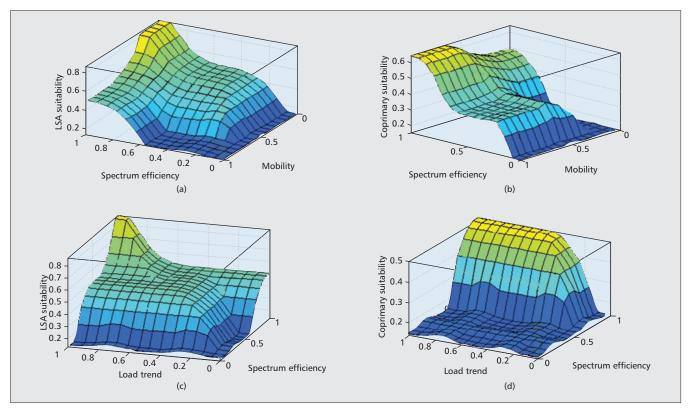
Figure 4. LSA and co-primary spectrum sharing suitability: a) LSA suitability in relation to spectrum efficiency and average user mobility; b) co-primary suitability in relation to spectrum efficiency and average user mobility; c) LSA suitability in relation to load trend and spectrum efficiency; d) co-primary suitability in relation to load trend and spectrum efficiency;
