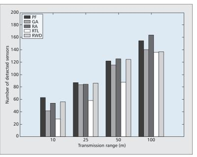
Figure 6. Number of detected sensor nodes for various mobile sink mobility models with varying transmission ranges.
