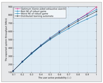
Figure 8. The expected Shannon capacity when varying the active probabilities of the cells.
