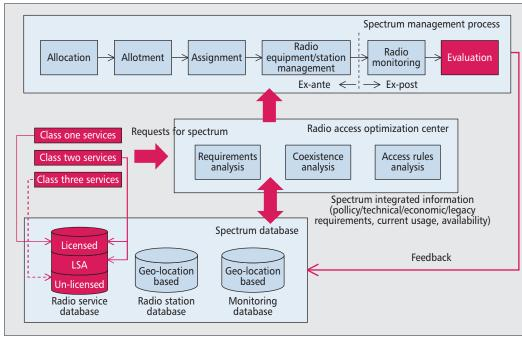
When a new service access request arrives, the center checks the database, performs integrated analysis, and outputs the solution to support the process, which conversely inputs the information to the database for further use, establishing a closedloop management.
