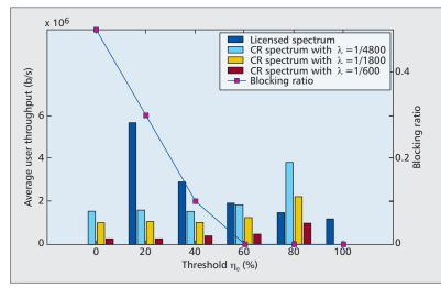
Figure 5. Average unblocked user throughput on licensed spectrum and cognitive spectrum.
