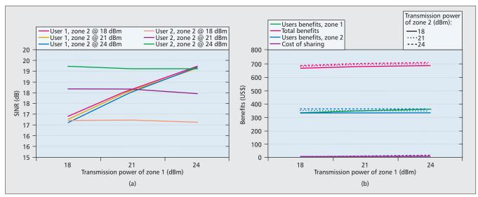
Figure 5. a) Achieved average SINRs for the sets of users in Scenario 3, against varied transmission power; and b) profits of the two sharing operators, individually and combined.
