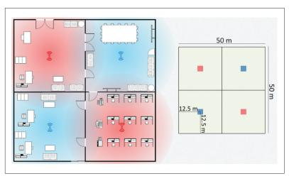
Figure 3. Indoor inter-operator deployment scenario. Different colors represent BSs of different operators.
