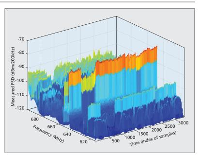
**Figure 1.** The 3-D view of the evolution trajectories of one week real-world RSS in the TV bands (614~698 MHz). For each 200 kHz spectrum band, about 3360 samples one week and thus 480 samples one day are plotted.
