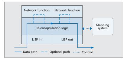
Figure 3. LISP re-encapsulating tunnel router.
