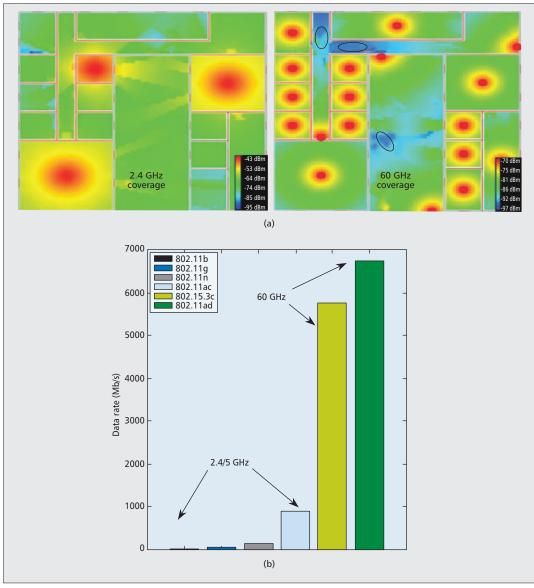
Almost every consumer electronic device, such as smartphones, tablets, laptops, cameras, etc., is equipped with WiFi and this trend is expected to continue. Hence, assistance of the 2.4/5 GHz band for 60 GHz communications seems a pragmatic solution.
