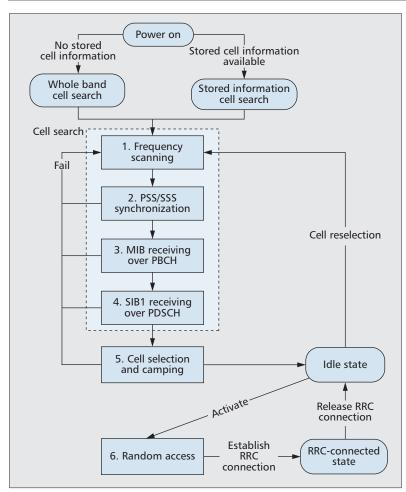
Figure 1. Network access in LTE networks.
