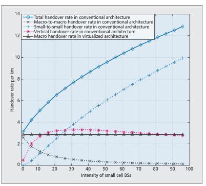
Figure 5. The handover rate per km for conventional and virtualized network architecture, the curve is plotted via stochastic geometry analysis following the footsteps of [15].
