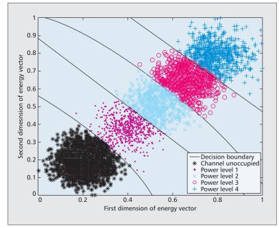
Figure 4. Clustering results and SVM trained decision boundary on normalized energy feature vectors when average SNR is -12 dB.
