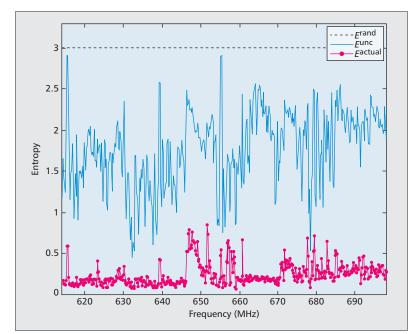
**Figure 3.** The entropy of the RSS dynamics in TV bands. The number of RSS levels is set as Q = 8 for each individual 200 kHz spectrum band and thus the random entropy  $E^{\text{rand}} = \log_2(Q = 8) = 3$  bits.
