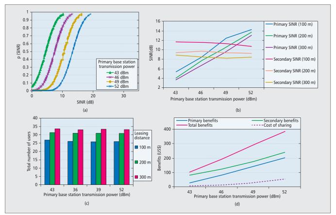
**Figure 3.** Results achieved for the first scenario: a) cumulative distribution function of the average SINR; b) averaged SINR observed by the primary and secondary users as the function of the leasing distance and transmit power; c) average number of supported users; d) financial benefits.
