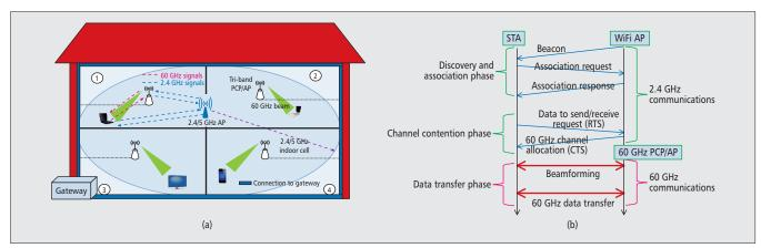
**Figure 3.** Interplay of 2.4 GHz and 60 GHz frequency bands in the proposed indoor network in 5G: a) network architecture; and b) sequence diagram of dual band transmission.
