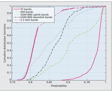
Figure 5. The cumulative distribution functions (CDFs) for the predictability of various services.
