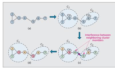
Figure 6. An example of using "divide-and-conquer" to use cluster-based hierarchical game in large-scale CSCs. In c) and d), the colors represent the channels chosen by the small cells.
