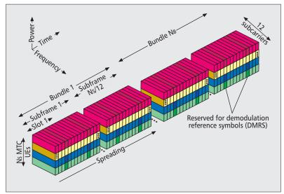
Figure 1. Structure of the bundling and spreading blocks for flexible TTI bundling and CDMA in PUSCH. Spreading with length  $N_S$  is performed over one or more consecutive sub-frames, which form a "spreading bundle." The spreading bundle is repeated  $N_B$  times. Calculation and assignment of  $N_B$ ,  $N_S$ , and code index to MTC UEs is done by a scheduling protocol in the eNodeB.
