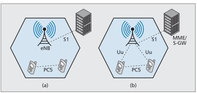
Figure 1. Architecture of a) D2D-unaware; b) D2D-aware LTE cellular networks.
