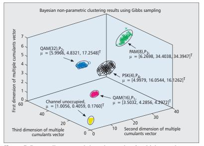
**Figure 5.** Pattern discovery and clustering results of multiple cumulants vectors before normlization using the DPGMM.  $\mu$  denotes the mean vector of each Gaussian component, and  $P_i$  denotes the transmit power level where  $P_1^2: P_2^2: P_3^2: P_4^2 = 2.5: 5: 5.3: 4$  when overall average SNR is 10 dB and the number of samples is 100.
