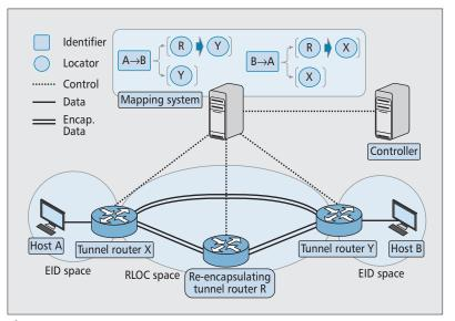
Figure 5. LISP SDN prototype.
