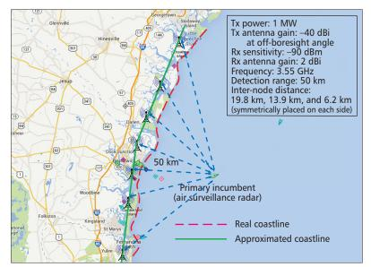
Figure 3. Illustration of sensor placement for incumbent detection and simulation context.
