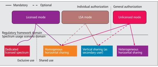
Figure 3. Illustration of spectrum type and related usage scenarios.
