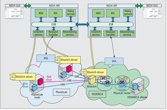
Figure 1. NOVI data, control, and management architecture.
