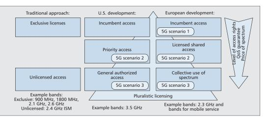
Figure 1. Pluralistic licensing in the context of spectrum sharing approaches for 5G.
