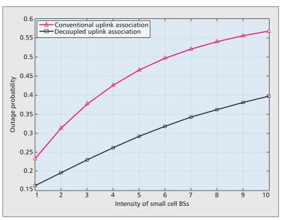
**Figure 3.** Outage probability vs small-cell intensity for virtualized and conventional cellular architecture, the curves are obtained via stochastic geometry analysis following the footsteps of [14].
