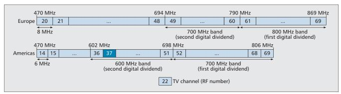
Figure 1. Frequency allocations in the UHF band for digital terrestrial broadcasting in ITU Region 1 (Europe, Middle East and Africa, and Russia) and Region 2 (Americas).
