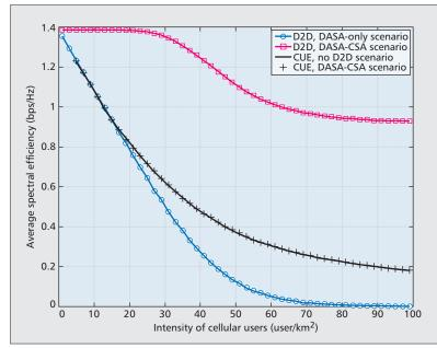
**Figure 4.** Spectral efficiency of transmission in D2D links vs. spatial intensity of cellular users for DUSA and DASA policies (with and without cognition).
