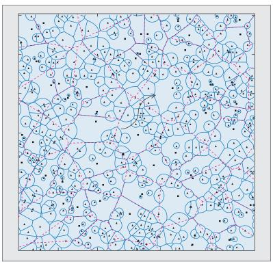
**Figure 4.** A two tier cellular networks with macro-BS (squares), small-cells (triangles), and a user's trajectory (highlighted in black). The figure shows the handover boundaries (in blue) for the conventional cellular network architecture and handover boundaries (in dotted red) for the virtualized cellular network architecture.
