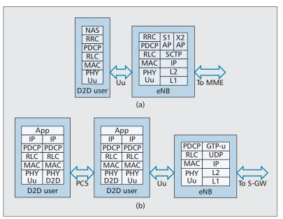
Figure 2. Protocol stacks for D2D-enabled LTE networks: a) control plane; b) user plane.
