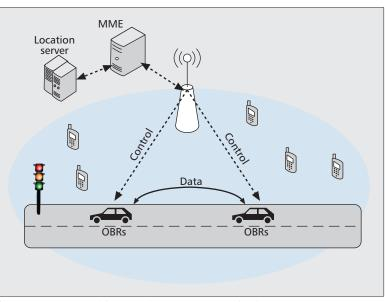
Figure 2. Access architecture for V2V communication.
