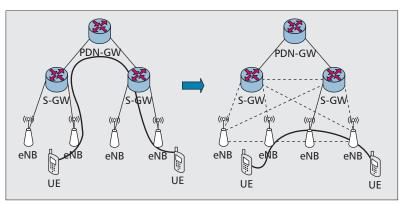
Figure 4. Example of route optimization in an EPS network.
