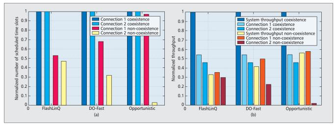
Figure 4. Experimental results: a) number of scheduled time slots; b) throughput comparison.
