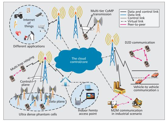
It is worth noting that centralized network control in the cloud does not necessarily mean a centralized execution for network functionalities. Some network functions may be implemented in a distributed cognitive manner while the cloud only dictates the operational quidelines.
