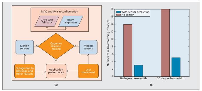
Figure 5. Sensor-assisted intelligent beamforming: a) system diagram of sensor assisted beamforming; b) re-beamforming instances.
