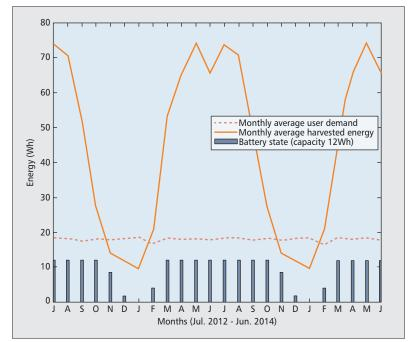
**Figure 4.** Average daily harvested energy and user demand aggregated over a month and the corresponding average battery state.  $\lambda_U$  (user density) =  $6\lambda_M$  (metro-cell density),  $\alpha = 4$ ,  $\lambda_{LP} = 0.48 \times 10^{-3}$  (Nottingham City) and  $\sigma^2 = -90$  dB/Hz.
