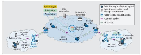
Figure 3. Illustration of the interactions between the QoE-controller and the various QoE data sources.
