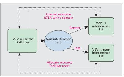
Figure 7. Sensing algorithm flowchart.
