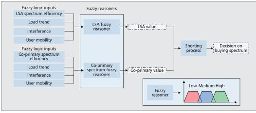
Figure 3. Fuzzy Logic based spectrum controller.
