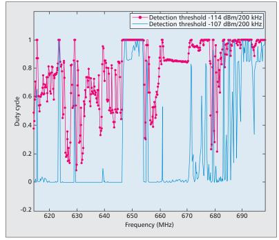
Figure 2. Impact of the detection threshold on the duty cycle in TV bands (614~698 MHz).
