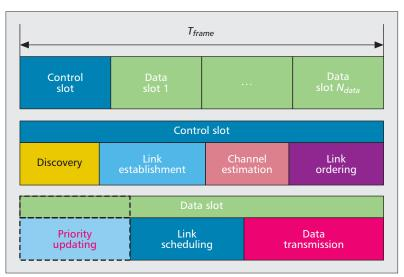
**Figure 1.** Frame architecture of the proposed scheduling mechanism in overlay mode.
