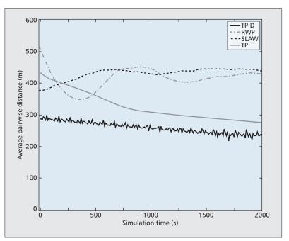
Figure 5. Average pairwise distances by simulation time for TP-D, TP, SLAW, and RWP models.
