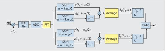
Figure 6. Cyclostationary detector of OFDM signal.
