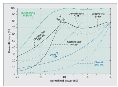
Figure 2. Ideal drain-efficiency characteristics of several high-efficiency amplifiers: (assuming class-B branch amplifier operation) two-way symmetric and asymmetric Doherty amplifiers (D-PA) [2], LINC (Fig. 1d) [2, 3], and outphasing with only phase modulation (PM-PA) [1, 2, 4] or using a combination of amplitude and phase modulation (i.e., mixed-mode outphasing) (MM-PA) [5]; and pure switch-mode outphasing with class-E branch amplifiers (E-SMPA) [6].
