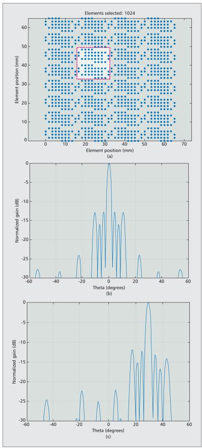
**Figure 5.** a) Array simulation with 1024 isotropic radiation elements based on the 94 GHz package antenna pattern (as highlighted); b) simulated 1024-element radiation pattern ( $\theta = 0^{\circ}$ ); c) simulated 1024-element radiation pattern ( $\theta = 30^{\circ}$ ).
