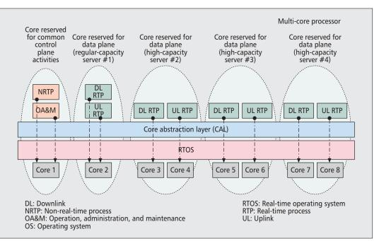
Figure 3. Deterministic symmetric multi-processing (D-SMP) configuration.
