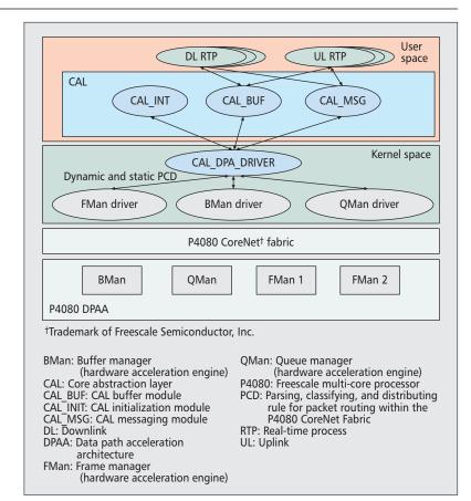
Figure 4. Core abstraction layer functional architecture.
