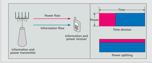
Figure 1. Model and protocol for combined case of SWIPT.
