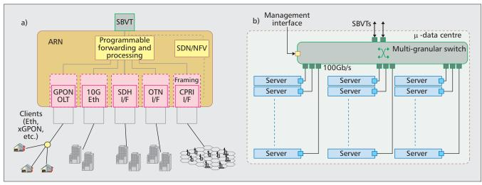
Figure 2. SHINE's ARN (a) and  $\mu$ -DC (b) architecture.
