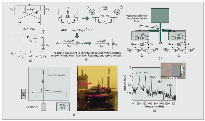
**Figure 4.** a) Conventional negative resistance generation mechanisms that introduce extra capacitance; b) the working mechanism of the proposed frequency-selective negative resistance tank; c) the complete terahertz generation circuit with fourth order harmonic enhancement by double push-pull scheme; d) the Michaelson interferometer measurement setup; e) the measured output spectrum with die photo shown in inset.
