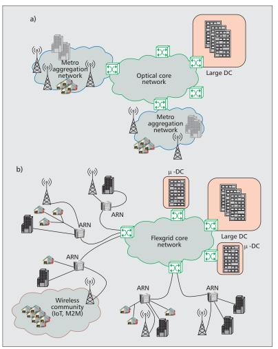
Figure 1. a) Current and b) SHINE network scenario. SHINE combines hybrid access and a distributed DC connected through a flexgrid core network.
