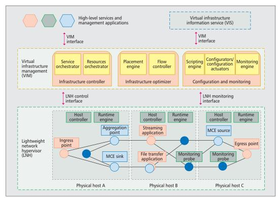
Figure 3. The Virtual Infrastructure Management and the Lightweight Network Hypervisor.
