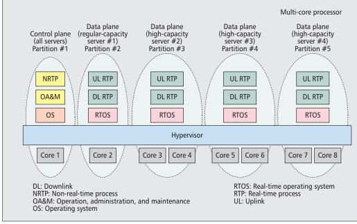
Figure 1. Supervised asymmetric multi-processing (S-AMP) configuration.
