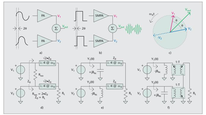
**Figure 1.** Outphasing amplifier topologies: a) analog; b) digital; c) signal vector representation of an outphasing amplifier. Examples of typical power combiners: d) an isolating Wilkinson power combiner; e) non-isolating transmission line-based combiner; f) transformer-based combiner.
