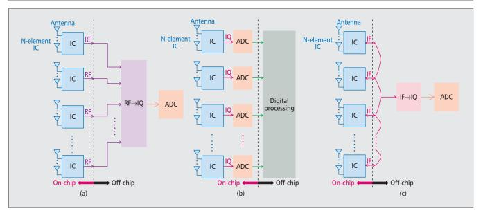
Figure 2. Scalable array system architecture concepts: a) distributing RF signals from IC output; b) digital beamforming; c) distributing IF signals between daisy-chained unit cells.
