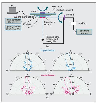
Figure 6. a) Radiated power and pattern measurement setup; b) measured 64-element array radiation patterns and beam steering.
