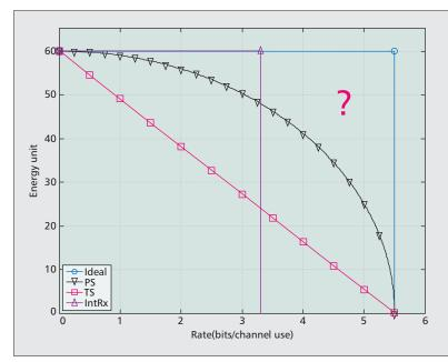
Figure 5. Comparison of rate-energy trade-offs of SWIPT receivers.
