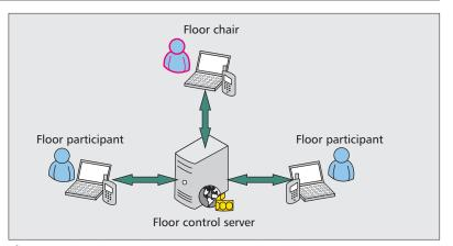
Figure 1. The Binary Floor Control Protocol architecture.
