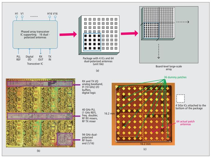
Figure 4. a) A prototype scalable 64-element phased array at 94 GHz; b) dual-polarized 16-element 94 GHz phased array transceiver IC photograph (6.6 mm  $\times$  6.7 mm); c) a close-up view of the 4-chip package with actual patch antennas and dummies.
