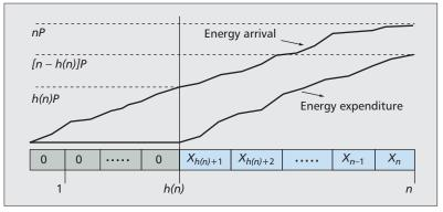
Figure 4. The code symbol energy expenditure and cumulative energy arrival curves in the save-and-transmit scheme.
