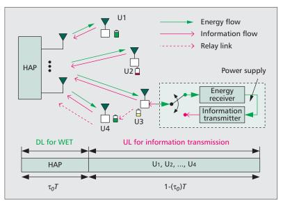
Figure 6. A WPCN model and the harvest-then-transmit protocol.
