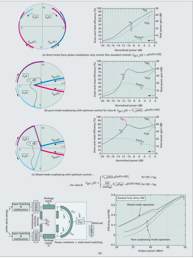
Figure 3. Outphasing using class-B branch amplifiers with different drive profiles [11, 12]: response of a) direct brute-force phase modulation only control; b) pure-mode; c) mixed-mode outphasing operation with ideal control for class-B operation. A practical class-B prototype schematic and corresponding measured results are given in d) for both pure-mode and mixed-mode operation [5].
