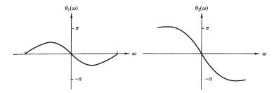
Minimum-phase:  $\angle H(\pi) - \angle H(0) = 0$ ; Maximum-phase:  $\angle H(\pi) - \angle H(0) = \pi$ .
