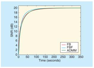
[FIG9] The SNR as a function of the computation time using ADMM and FB- or FBF-based primal-dual methods for a given slice. The MATLAB implementation was done on a 2.9-GHz Intel i7-3520M central processing unit (CPU).
