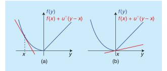
[FIG2] Examples of subgradients u of a function f at x.
