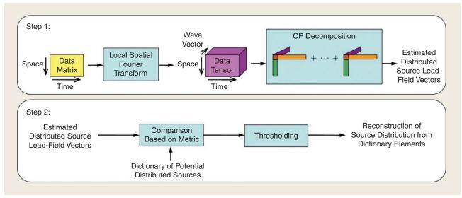
[FIG3] A schematic representation of the STWV-DA algorithm.
