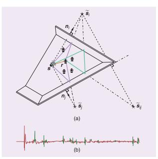
[FIG10] (a) An illustration of the IS model for first- and secondorder echoes. Vector  $n_i$  is the outward-pointing unit normal associated with the *i*th wall. The stars denote the IS, and  $\tilde{s}_{ij}$  is the IS corresponding to the second-order echo. The sound rays corresponding to first reflections are shown in purple, and the ray corresponding to the second-order reflection is shown in green. (b) The early part of a typical recorded RIR.
