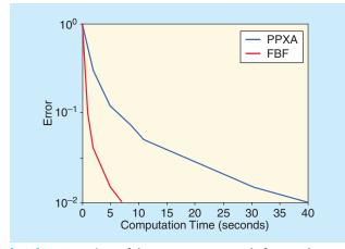
[FIG7] A comparison of the convergence speed of a Douglas– Rachford-based algorithm (PPXA [65]) (blue) and an FBF-based primal–dual algorithm (red) for image denoising using a nonregular graph. The MATLAB implementation was done on an Intel Xeon 2.5-GHz, eight-core system.
