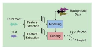
[FIG4] An overall block diagram of a basic speaker-verification system.
