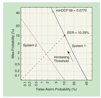
[FIG11] DET curves of two speaker-verification systems (System 1 and System 2). In System 1, the points on the curve corresponding to the threshold that yields the EER and minimum DCF (as in NIST SRE 2008), and the direction of an increasing threshold are shown. Being closer to the origin, System 2 shows a better performance.
