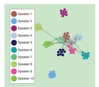
[FIG9] A graphical representation of 79 utterances spoken by ten individuals collected from the NIST SRE 2004 corpus. The i-vector representation is used for each segment; the plot is generated using GUESS, an open-source graph exploration software [123] that can visualize higher-dimensional data using distance measures between samples.
