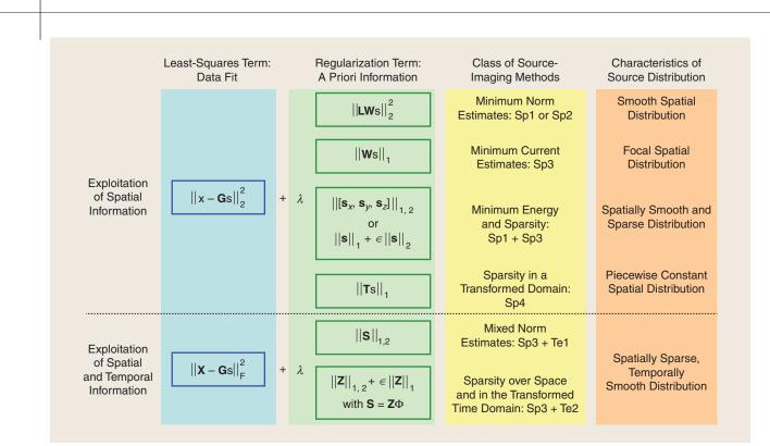
[FIG2] An overview of regularized least-squares algorithms. (For an explanation of the employed notations for the different algorithms, see the text in the associated sections.)
