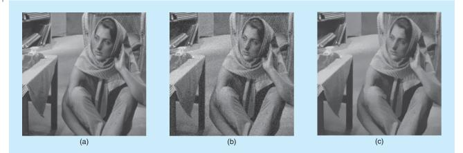
[FIG6] Nonlocal denoising (additive white zero-mean Gaussian noise with variance  $\sigma^2 = 20$ ): (a) original image, (b) noisy signal-tonoise ratio (SNR) = 14.47 dB, and (c) nonlocal TV SNR = 20.78 dB.
