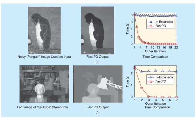
[FIG10] The FastPD [126] results for (a) an image denoising and (b) a stereomatching problem. Each plot in (a) and (b) compares the corresponding running time per iteration of the above primal-dual algorithm with the  $\alpha$ -expansion algorithm, which is a primal-based method (experiments conducted on a 1.6-GHz CPU).
