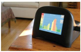
[FIG4] The Speck air-quality monitor allows users to view the level of fine particulate matter suspended in the air inside their homes. (Photo courtesy of Airviz, Inc.)
