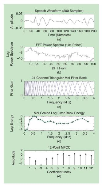
[FIG6] Steps in MFCC feature extraction from a speech frame: (a) 200-sample frame representing 25 milliseconds of speech sampled at a rate of 8 kHz, (b) DFT power spectrum showing first 101 points, (c) 24-channel triangular Mel-filter bank, (d) log filter-bank energy outputs from Mel-filter, and (e) 12 static MFCCs obtained by performing DCT on filter-bank energy coefficients and retaining the first 12 values.
