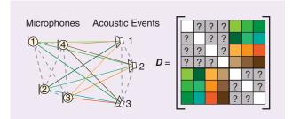
[FIG4] The microphone calibration as an example of MDU. We can measure only the propagation times from acoustic sources at unknown locations to microphones at unknown locations. The corresponding revealed part of the EDM has a particular offdiagonal structure, leading to a special case of EDM completion.
