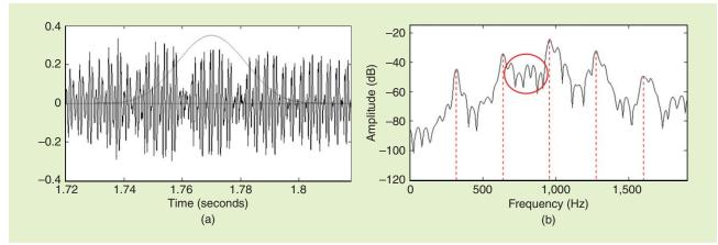
[FIG3] The growl analysis of a singing voice sample: (a) waveform and (b) spectrum with harmonics (dashed lines) and subharmonics (circle).
