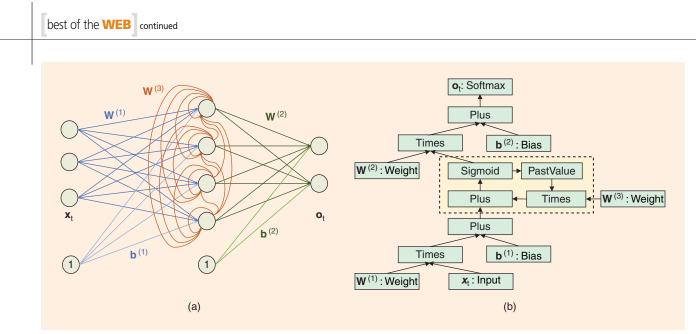
[FIG1] NN-CN representation correspondence for a single-hidden-layer neural network with a recurrent loop from the hidden layer to itself. Nodes of the CN are represented using the [node name]: [node type] or [node type] format. (a) Neural network representation. (b) CN representation.
