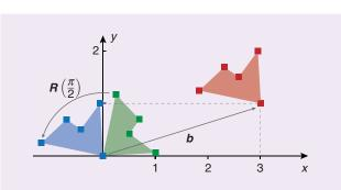
[FIG3] An illustration of a rigid transformation in 2-D. Here, the point set is transformed as  $RX + b1^{\top}$ . The rotation matrix  $R = [0 \ 1; -1 \ 0]$  (MATLAB notation) corresponds to a counterclockwise rotation of 90°. The translation vector is  $b = [3, 1]^{\top}$ . The shape is drawn for visual reference.
