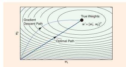
[FIG1] Mean trajectories of an ensemble of noisy single-realization gradient descent paths for correlated data. The LMS path, produced based on (9), is locally optimal but globally slower converging than the optimal path.
