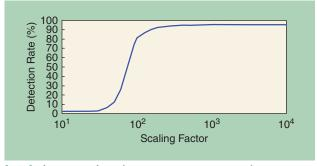
[FIG5] The correct detection rate versus representation accuracy in the face-recognition system described in [19].
