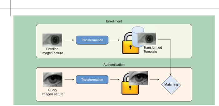
[FIG1] A block diagram of a cancelable biometric system.
