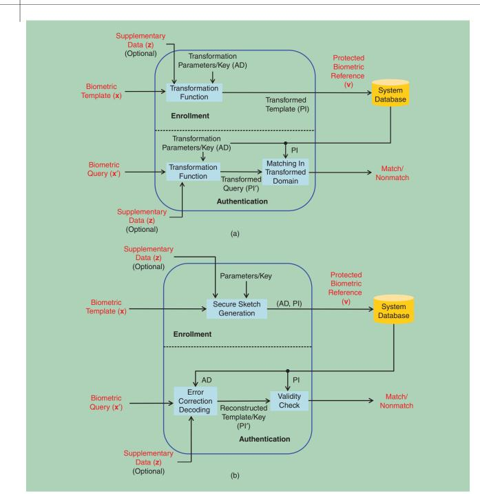
[FIG4] There are two broad approaches for biometric template protection: (a) feature transformation and (b) biometric cryptosystem. The protected biometric reference (denoted by v) generally consists of two distinct parts: pseudonymous identifier (PI) and auxiliary data (AD).
