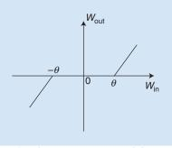
[FIG1] Soft-thresholding:  $w_{out}$  [n] = sign ( $w_{in}[n]$ ) max{( $|w_{in}[n]| - \theta$ ), 0}.
