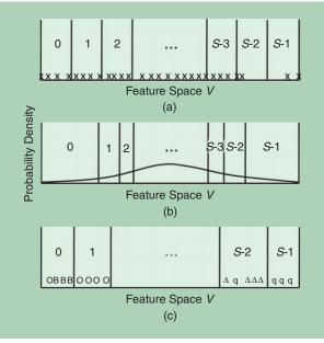
[FIG5] Illustrations of (a) equal width, (b) equal-probable quantization, and (c) entropy quantization, where "X" in (a) denotes unlabeled samples; probability density function in (b) denotes the population distribution; and "O," "B," " $\Delta$ ," and "Q" in (c) denote labeled samples from four different classes.
