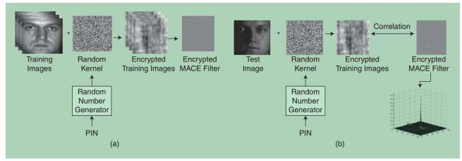
[FIG4] A correlation filter-based approach to cancelable biometrics [23]. (a) The enrollment stage for encrypted filters. (b) The authentication stage using encrypted MACE filters.
