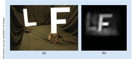
[FIG2] A regular photograph of cardboard cutout letters and the reconstructed indirect image captured by the modified Creative Senz3D camera.
