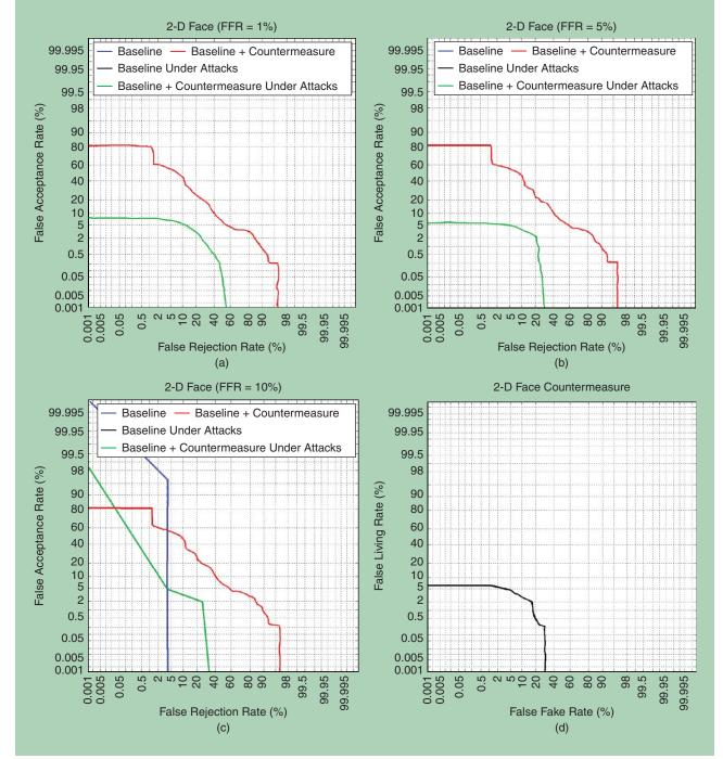
[FIG12] DET profiles for the 2-D face verification systems with/without spoofing and with/without countermeasures at different countermeasures operating points [FRRs of (a) 1%, (b) 5%, and (c) 10%]. Missing profiles indicate EER = FRR = FAR = 0%. Also illustrated in (d) is a DET profile for the independent countermeasure.
