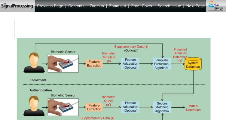
[FIG2] The general framework of a biometric system with template protection.
