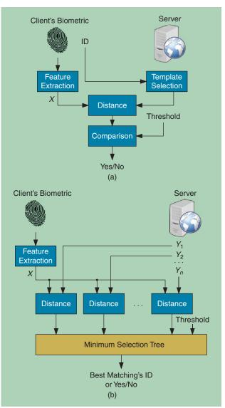
[FIG1] Biometric recognition protocols: (a) authentication and (b) identification.
