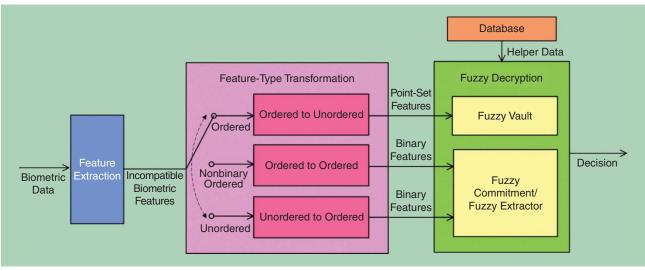
[FIG1] A generic biometric cryptosystem with feature-type transformation.
