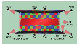
[FIG2] An image from the Southampton Multi-biometric Tunnel [8]. The tunnel automatically recognizes individuals passing through it using three-dimensional gait, ear, and face recognition. Such systems can have many applications but also raise significant privacy concerns as they have the potential to be deployed covertly.
