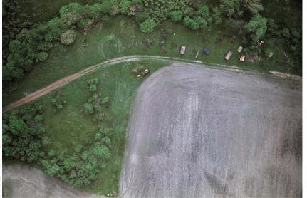
[FIG4] Image enhancement allows the extraction of additional details within the target area, enabling the automated surveillance technology to accurately detect and classify objects that pose a possible threat to a nearby pipeline.
