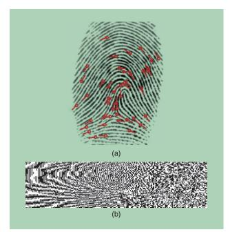
[FIG6] An example of embedding a point set as a binary string. (a) Fingerprint with minutiae (point set) marked on it and (b) the corresponding binary string representation obtained using the binarized phase spectrum technique [34].
