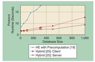
[FIG2] The runtime comparison of HE [19] and hybrid [25] implementations of the eigenface protocol.
