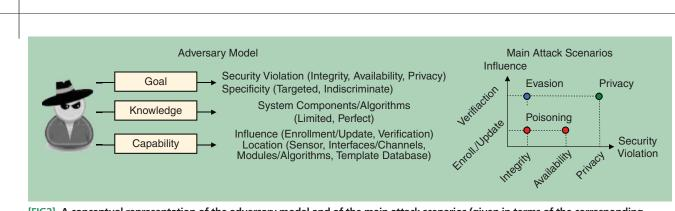
[FIG2] A conceptual representation of the adversary model and of the main attack scenarios (given in terms of the corresponding security violation and attack specificity) according to our framework.
