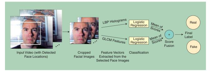
[FIG10] A block diagram of the texture-based countermeasure.
