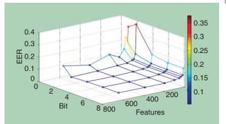
[FIG6] The EER of the different configurations of fingercode [33] on the fingerprint database [43].
