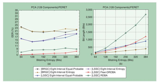
[FIG7] A comparison of ordered continuous-to-binary transformation schemes in (a) performance and (b) bit length of binary representation based on the FERET face data set.
