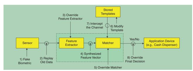
[FIG 8] Possible attack points in a generic biometric system [8], [46].
