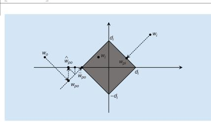
**[FIG2]** A graphical illustration of s projection onto an  $\ell_1$ -ball with size  $d_i$ : Vectors  $w_{pi}$  and  $\tilde{w}_{po}$  are orthogonal projections of  $w_i$  and  $w_o$  onto an  $\ell_1$ -ball with size  $d_i$ , respectively. The vector  $w_i$  is inside the ball,  $||w_i||_1 \leq d_i$ , and projection has no effect:  $w_{pl} = w_l$ .
