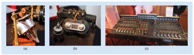
[FIG2] The EMI Archive Collection. (a) A Blumlein-pair ribbon microphone consisting of two colocated microphones oriented at 90° to one another. (b) A stereo cutting tool to record two audio channels in a single grove of a vinyl disk. (c) A mixing desk of the 1970s (TG 12345 Mk II) indicating the complexity that audio engineers faced to combine several sources and produce a professional-quality audio recording track.
