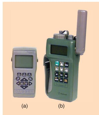
**[FIG2]** (a) The next-generation version DAGR of the (b) Precision Lightweight GPS Receiver (PLGR). (Image courtesy of Rockwell Collins and used with permission.)
