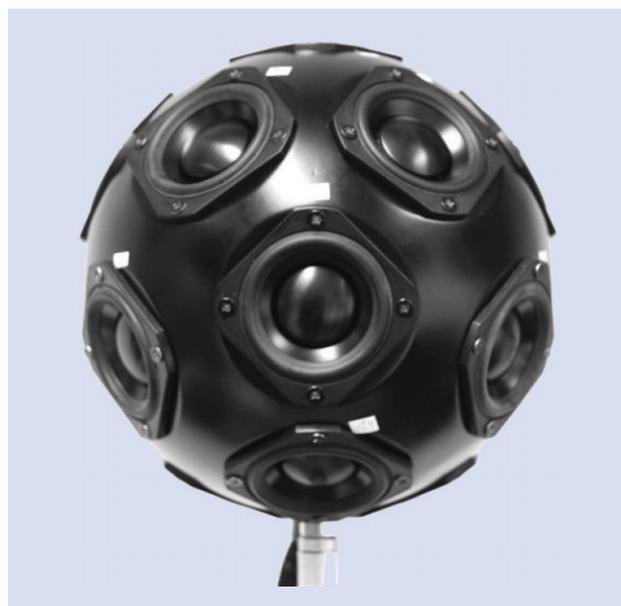
**[FIG4]** A spherical array of loudspeakers (figure used with permission of [30]).
