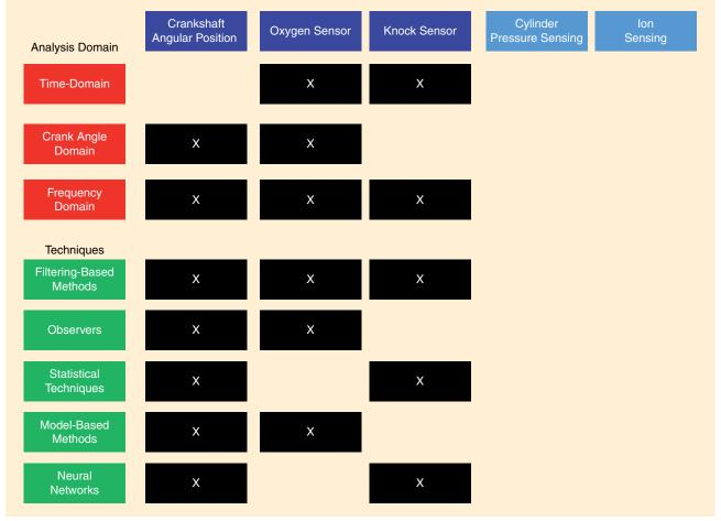
FIGURE 1. The taxonomy of DSP applications in engine controls and diagnostics.
