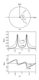
A resonant peak at or near  $\omega = \omega_0$ ,
