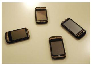
FIGURE 3. An ad hoc array composed of smartphones. (Photo used courtesy of TU Dortmund.)
