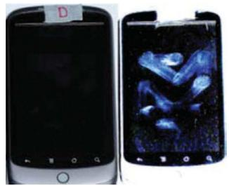
FIGURE 1. A smudge attack [3]. A user's secret pattern can be determined with special lighting and high-resolution camera.
